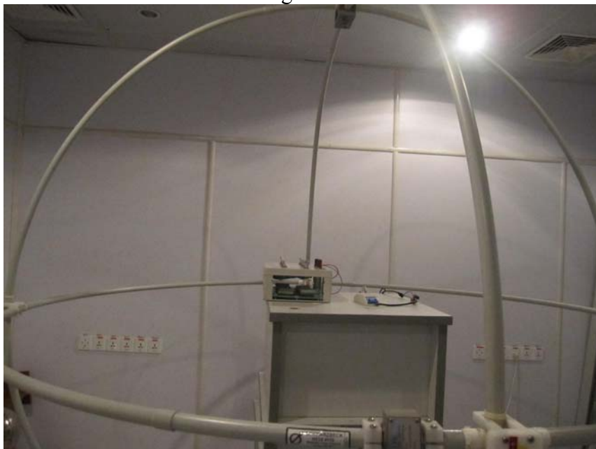
Radiated Electromagnetic Filed Disturbance
